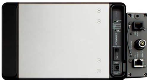
Figure 1: Voyager 2 rear showing UBI-2590 battery, DC input and HAiPE power
